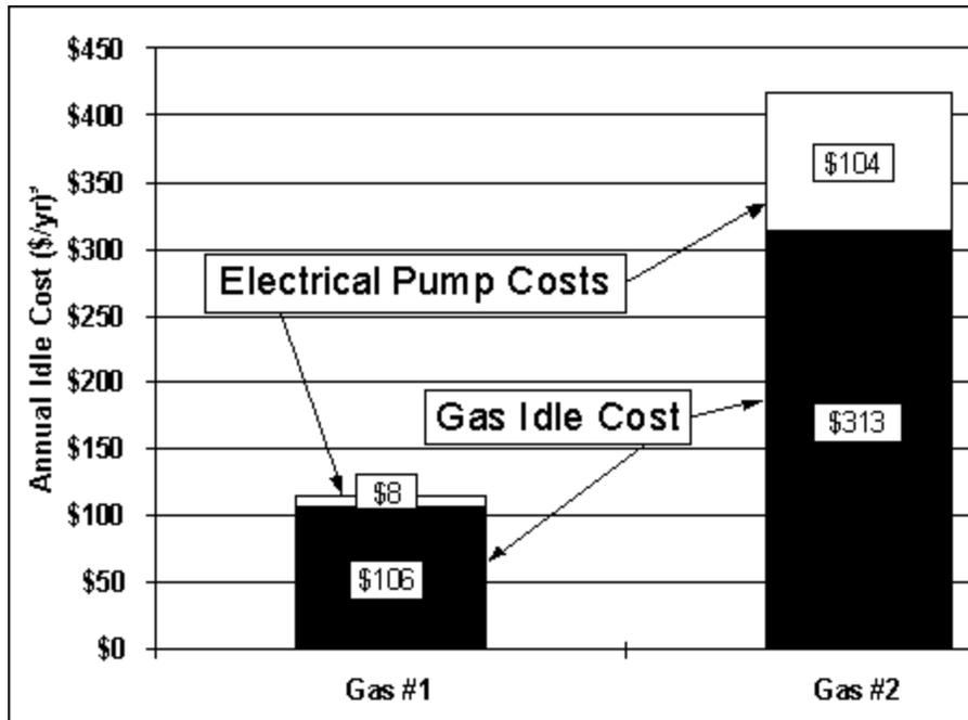
**Graph 1. Gas Booster Heater Idle Performance Characteristics**
